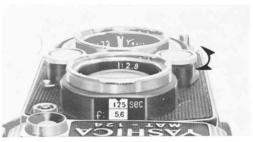
② Center the desired shutter speed in the Shutter Speed Indicator Window by turning the Shutter Speed Control Dial. The exposure meter pointer in the Exposure Indicator Window is coupled to the shutter mechanism and will shift in either direction when the shutter speed is adjusted.
