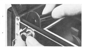
•To minimize the trouble in loading your next film, it is advisable to take out the empty spool from the lower film chamber and to set it in the upper chamber immediately after unloading the exposed film.
