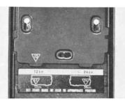
③ When loading a 120 film (12 exposures), position the green 127 mark on the film pressure plate so that it aligns precisely with the green 12 EX indication. Set the pressure plate so that its hole (C) rests properly on the stud and slide it toward the smaller side of the twin hole to mount it in position.
