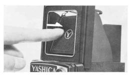
Your YASHICA-MAT 124 features a magnifying lens for critical focusing which springs up into position when the sportsfinder frame section of the Focusing Hood is pushed in slightly.
