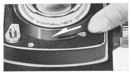
When using the self-timer, always see to it that the Flash Synchronizer Selector is switched to "X" position.
