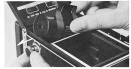
[3] Pull out the Upper Spool Holder Knob and take out the exposed film from the film chamber. Paste the seal to prevent recoiling and wrap the film in light-proof paper.
