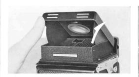
3 The exposure meter begins to function when the focusing hood is set upright by lifting it up gently with your fingertip.
