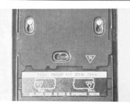
When loading a 220 film (24 exposures), align the red with the red 24 EX indication and mount it in position in the same manner as explained above.
